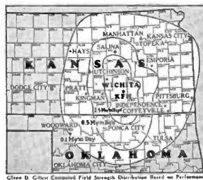
Green D. Gillett Compiled Field Strength Distribution Based on Performance and Previous Survey Measurements—5000 Watts Day and Night—October 1941
